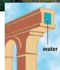
This is a photo of a Roman aqueduct in modern Spain that has survived. The cross section shows how the water moved within the aqueduct.
